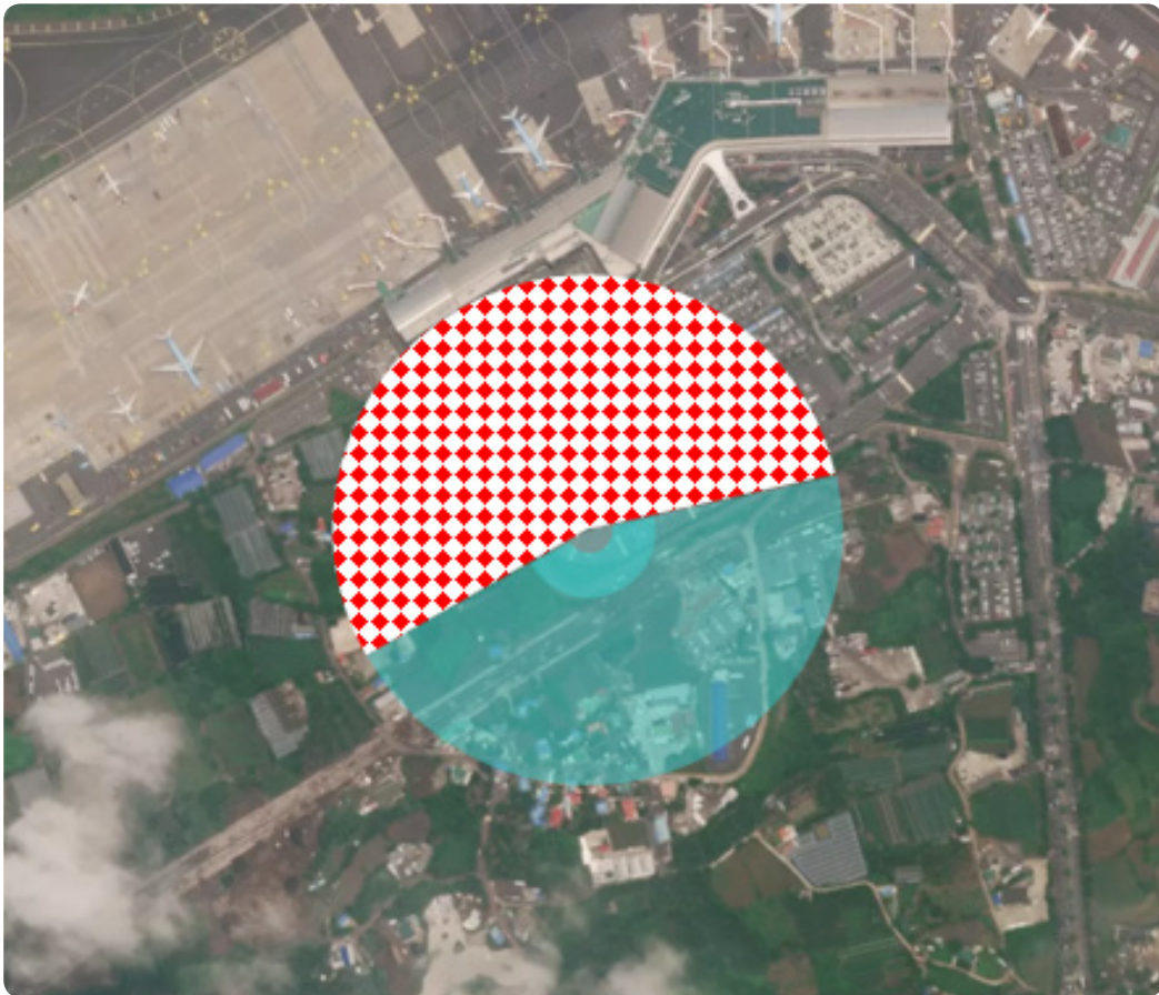
Possible Jeju Airport vertiport obstacle-free volume with omnidirectional approach and take-off climb surface and prohibited sector (top view). Source: Eve Air Mobility
