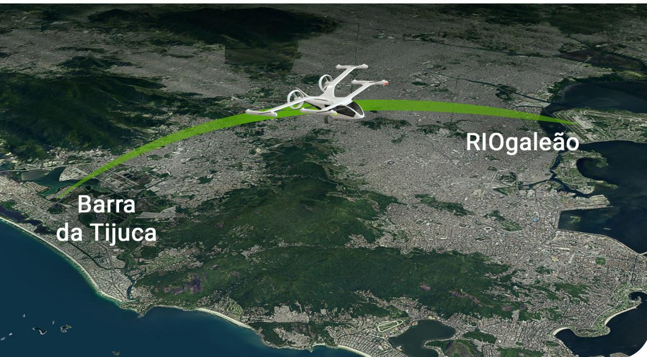
This CONOPS is based on an airport shuttle Use Case. It focuses on the trip between Barra da Tijuca and the Rio de Janeiro International Airport (Tom Jobim/Galeão). This 35-km drive can take about 1h30min or more by car, but, when considering a UAM flight, it can be completed in about 12 minutes, using the current helicopter corridors (Figure 10).
